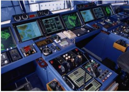
But new technical developments and integrated bridges have side effects on the use of basic radar. Video processors take time to build up a smooth picture; the radar screen is not necessarily placed under the antenna. Large vessels have radar antenna's on bow and one the stern of the vessel. That Radar information is transferred to a reference point:
